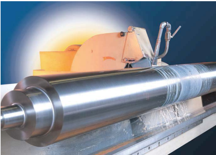
Final process in which repaired roll is receiving a standard mirror finish.
