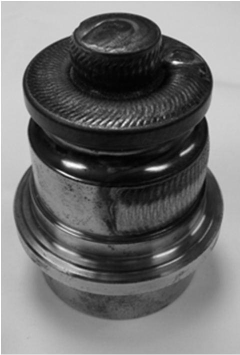
Figure 2. Rock Bit Journal Overlaid with Stellite 190 Crack Free
