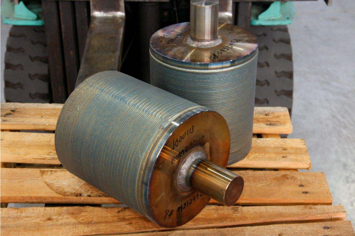
Figure 1. Nitronic 50 Overlaid with Stellite 6 crack free.
